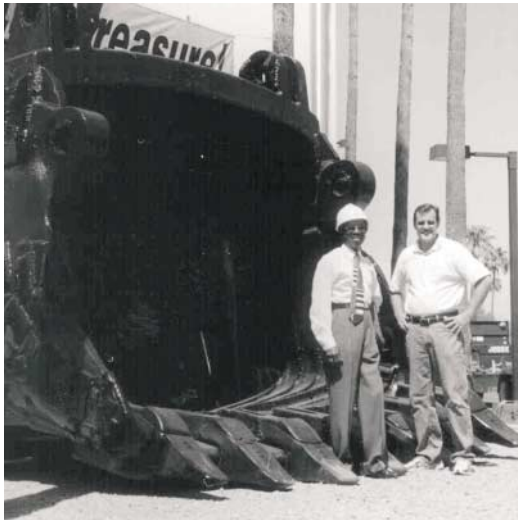
Ben Daniels (left) of APS and Doug Sawyer, Director, celebrate the successful delivery of the shovel bucket from the Ray mine. APS sandblasted and coated the bucket for the Department. The 100,000-pound bucket has already become a favorite with visiting school children.
